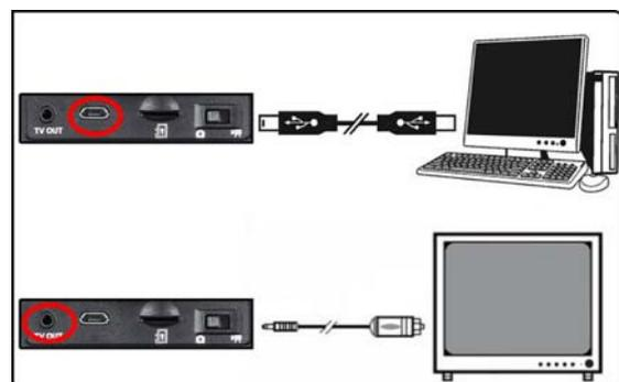
**9, TV OUTPUT JACK:** the “live” image as seen on the unit’s display is output here. Connect the included video cable between this jack and a video monitor or recorder to remotely view or record the image from the night vision unit.
